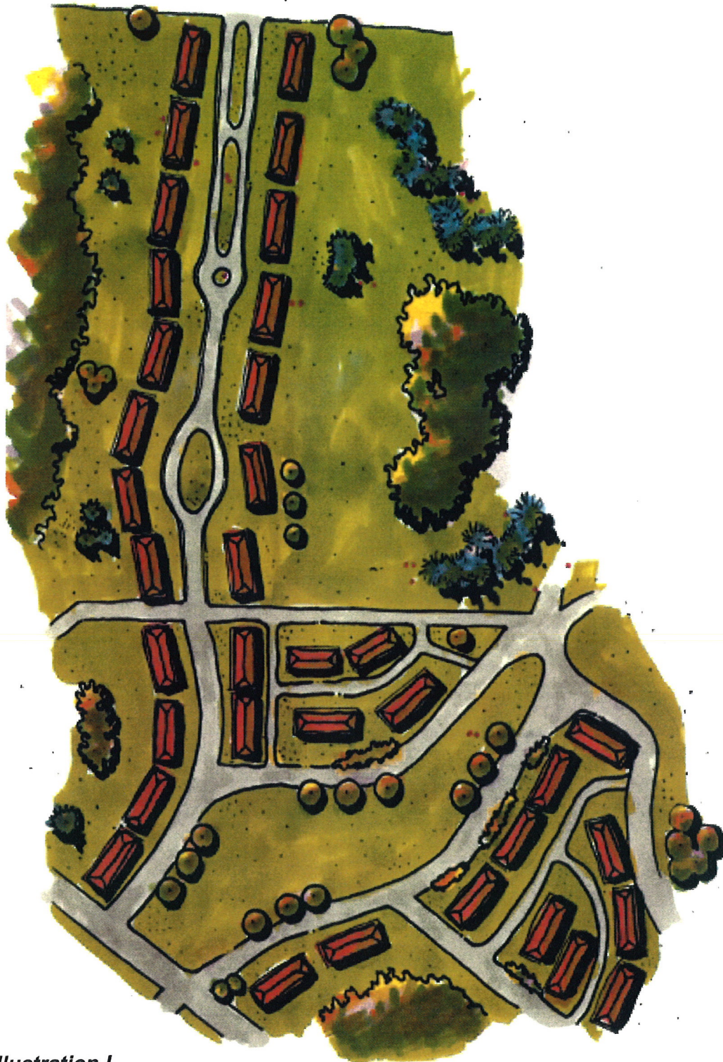
Illustration L This design transitions from a formal linear streetscape to townhomes clustered around a central park.
